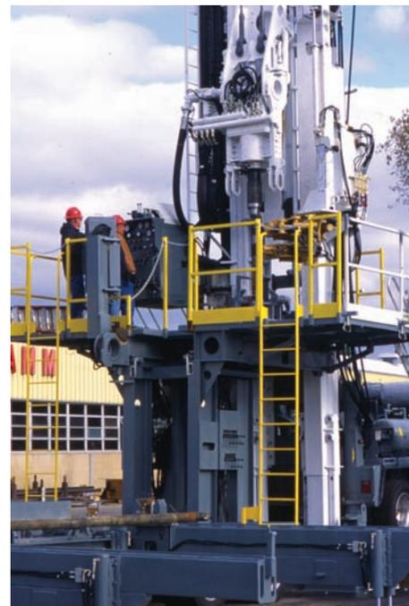
transporting the T130XD, the mast's overhang at the front of the rig's chassis is less than 6 ft. Since the TXD is trailer-mounted, an overhang is non-existent. Dave Wilson, superintendent for Whipstock, said the telemast tower is the single most outstanding feature to be found on the T130XD.
